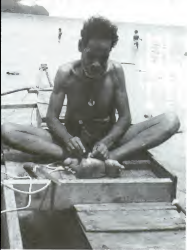
24. Zacharias making a fishhook from steel wire using a rock as an anvil. Chapter 9
