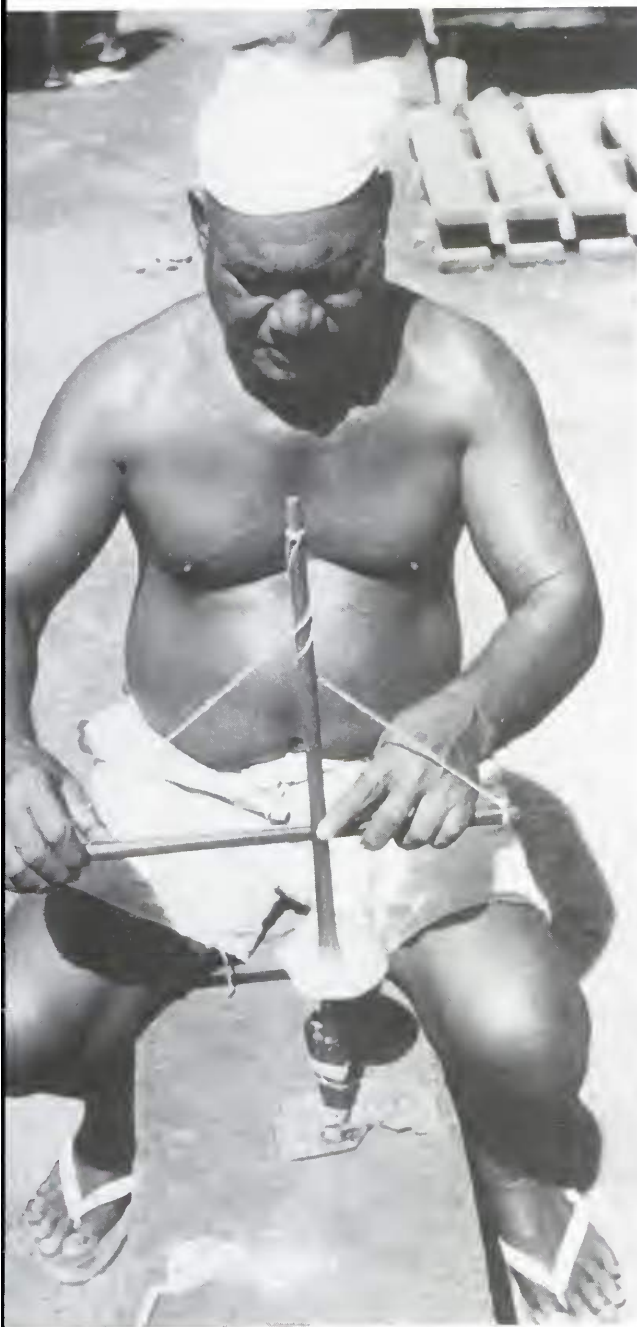
22. Kalisto demonstrating the device for cutting fishhook blanks. Chapter 9
